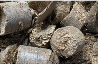
Briquette fuel made from highly compressed wood chips
