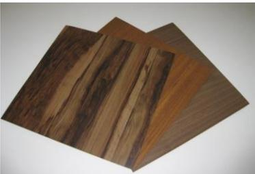
■ **Develop high pressure laminates (HPL) produced out of plant-based phenolic resins**
